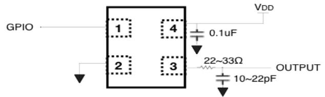
Non-modulated clock output when GPIO=Low
