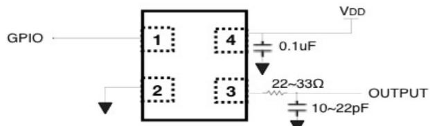
Non-modulated clock output when GPIO=High
