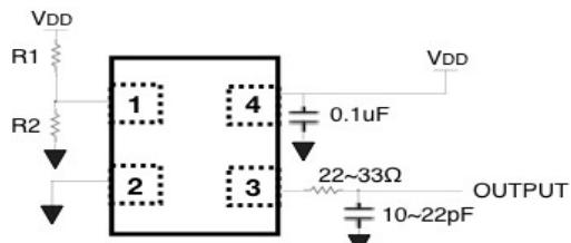
Non-modulated clock output when R1=NC or 4.7K, R2=NC
