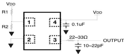
Non-modulated clock output when R1 = NC or 4.7KΩ , R2 = NC
