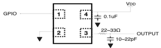
Non-modulated clock output when GPIO = High
