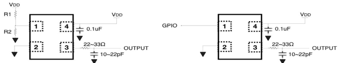
Non-modulated clock output when  $R1 = NC$  or  $4.7K\Omega$ ,  $R2 = NC$
